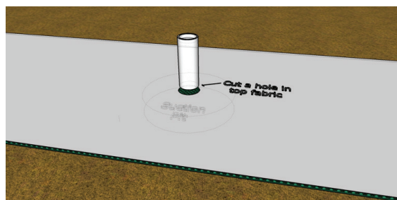
Figure 3: Vent Stack Installation
