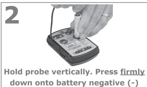
**Remember, press the probe tip firmly down onto the battery during the entire Pulse Load test (while LEDs are 'running').**
